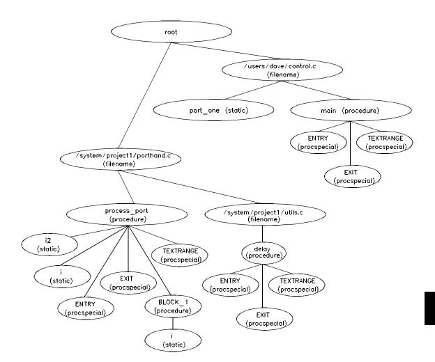
Note that SRU does not build tree nodes for variables that are dynamically allocated on the stack at run-time, such as i and j within the delay () procedure.
