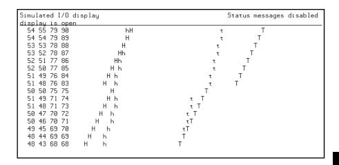
A message tells you whether the display is open or closed. You can modify the configuration to enable status messages.
