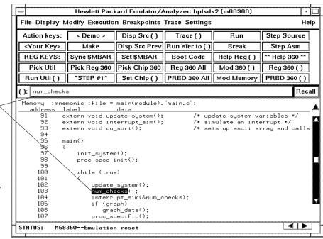
A mouse click causes the interface to expand the highlight to include the symbol "num\_checks" and paste the symbol into the entry buffer.
