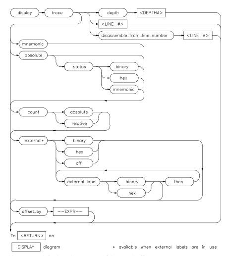
This command displays the contents of the trace buffer.
