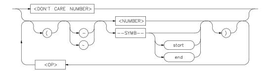
An expression is a combination of numeric values, symbols, operators, and parentheses used to specify address, data, status, executed address, or any other value used in the emulation commands.
